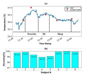
Figure 3: In-Ear thermometer performance evaluation. (a) In-Ear thermometer measured temperature in various conditions; (b) In-Ear thermometer accuracy across subjects.
